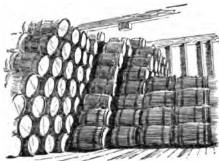
2411. The piling of barrels of apples in a cold storage house.
